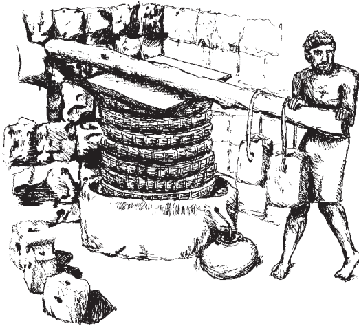
Olive mill grinding the ripe olives and producing “virgin” oil, and olive press with bags of smashed olives pressed down by weights that release the oil to the jar at the bottom.
