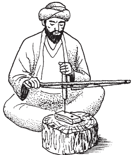
Carpenter with bow drill sitting on the floor, using a section of a tree for his workbench, typical in ancient Israel, where tables and benches were rarely used until late in history.
